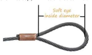
Soft eye diameter as standard is 15 x the wire rope diameter
